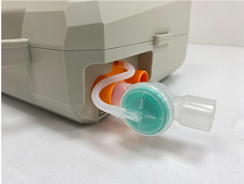
Figure 11 — Exhalation Valve Connection
