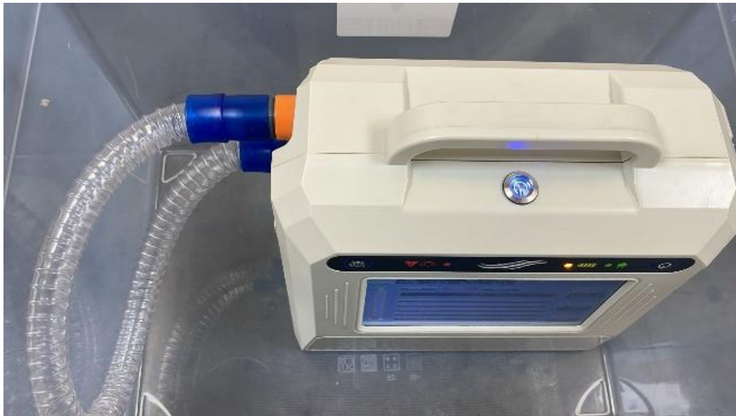
Figure 51—Ozone Generator Connection and Active Shocking
