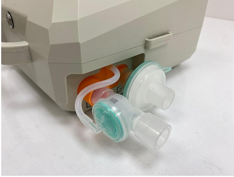
Figure 12 — Bacterial Filter and Patient Circuit
